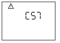
A three digit error code displays on the screen, indicating the type of error (e.g., error code 57 displays as C57). When a card error occurs, the BiPAP Synchrony's LCD backlight is turned on. Pressing either the **Reset** button or **Silence** button exits this screen and returns to the previous screen.
