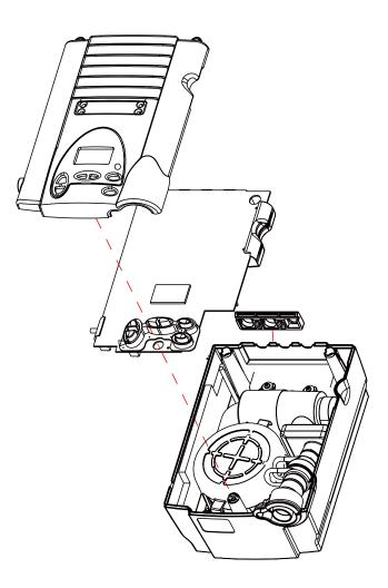
FIGURE C: REMOVAL AND INSTALLATION OF THE TOP ENCLOSURE
