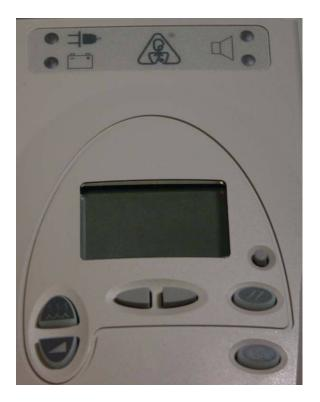
FIGURE A: BIPAP SYNCHRONY ALARM LEDS AND BUTTONS
