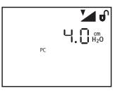
To change the ramp setting pressure, press the Heat and Ramp buttons until the correct pressure appears. The setting increases or decreases in 1.0 cmH<sub>2</sub>O increments. The user can adjust the setting from 4 cmH<sub>2</sub>O to the EPAP/CPAP pressure setting. Press the right user button to move to the next screen.
