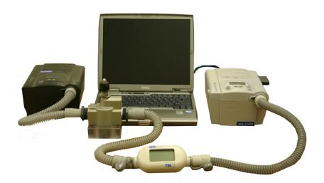
FIGURE W: SYSTEM CALIBRATION WITH NEGATIVE FLOW SOURCE
