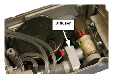
FIGURE M: DIFFUSER ASSEMBLY
