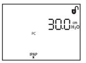
Increase or decrease the IPAP max pressure by pressing the Heat or Ramp buttons until the correct pressure appears. You can adjust the pressure from 4 to 30 cm  $H_2O$  in 1 cm  $H_2O$  increments. The IPAP max pressure setpoint cannot be set lower than the IPAP min pressure setting. Press the right user button to move to the next screen.
