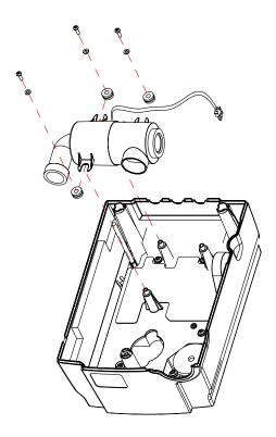
FIGURE N: REMOVAL AND INSTALLATION OF VALVE ASSEMBLY
