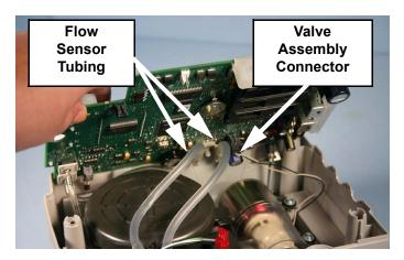
FIGURE H: FLOW SENSOR TUBING AND VALVE ASSEMBLY
