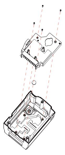
FIGURE R: REMOVAL AND INSTALLATION OF THE MUFFLER
