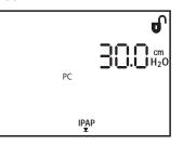
Increase or decrease the IPAP min pressure by pressing the Heat or Ramp buttons until the correct pressure appears. You can adjust the pressure from 4 to 30 cm  $H_2O$  in 1 cm  $H_2O$  increments. The IPAP min pressure setpoint cannot be set lower than the EPAP setting. Press the right user button to move to the next screen.
