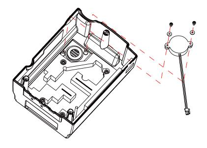
FIGURE S: REMOVAL AND INSTALLATION OF THE BUZZER ASSEMBLY
