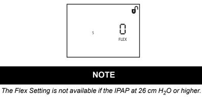
This screen allows you to adjust the level of air pressure relief that the patient feels when he or she exhales during therapy. To change the selection, press the Heat or Ramp buttons until the correct setting appears. The Flex set point is adjustable from 0-3 in increments of 1. Press the right user button to move to the next screen.
