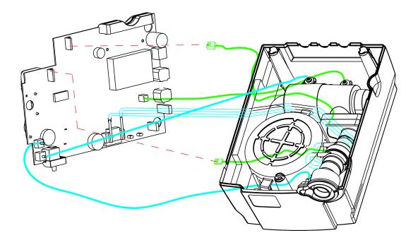
FIGURE E: REMOVAL AND INSTALLATION OF THE MAIN PRINTED CIRCUIT ASSEMBLY
