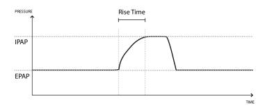
progressively reflect slowed response of the pressure increase that will take place at the beginning of inspiration. A setting of 1 is the fastest rise time while a setting of 6 is the slowest. Adjust the rise time to find the most comfortable setting for the patient. Rise time cannot be adjusted when Bi-Flex is enabled.
