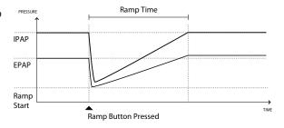
Max or Pressure Support Max. In AVAPS-AE mode, the EPAP will reduce to the EPAP Min setting but is not ramped, and Auto-EPAP adjusts the pressure according to the patient's needs. During the ramp period, the IPAP or pressure support applied will be adjusted by the AVAPS algorithm but will be constrained by the current maximum ramp pressure set point. The pressures (with exception of EPAP in AVAPS-AE mode) will then ramp up to the original prescribed settings over the ramp time period.
