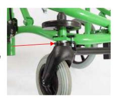
On the Small, there is a extra Washer. It has to stay on, when you mount the Leg separation plate.
