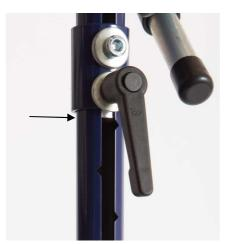
The height of the trunk support is altered by loosening the bottom two Allen screws and then the bottom two spanner grips. This enables the two rings to be slid up or down the upper tubes. Place the rings at the desired height using the height markings to ensure they are at the same height on both sides. At last retighten the spanner grips (and if necessary Allen screws).
