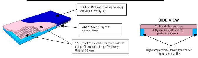
The LTC 3000 "Comfort Plus" mattress assists in providing pressure reduction, while ensuring that the patient receives a high degree of support. This high quality, high resiliency foam mattress is constructed with a 4" profile cut Ultracell 35 (2.75 lb density / 35 ILD) core and a 2" Ultracell 21 (2.5 lb density / 30 ILD) comfort layer topper. The LTC 3000 "Comfort Plus" has been specially designed for Acute Care where continuous usage is anticipated.
