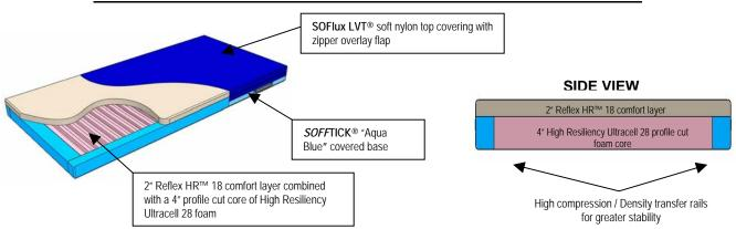
The LTC 4000 "Comfort Softee" uses a combination of premium, fire rated foam to provide exceptional comfort and support, while assisting in pressure reduction. This high quality, high resiliency foam mattress is constructed with a 4" profile cut Ultracell 28 (2.5 lb density / 30 ILD) core and a 2" Reflex HR™ 18 (1.8 lb density / 18 ILD) extra soft comfort layer topper. The LTC 4000 "Comfort Softee" mattress has been specially designed for Long Term Care.
