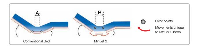
Compared to a conventional profiling bed (A), the *Pro-Contour Advance Profiling* on the four-section *Minuet 2* beds raises the pivot point of the backrest and thigh section closer to the client's natural pivot point (their hip joint) (B). As a client moves from a lying to a more upright position, this reduces abdominal compression, and improves comfort.
